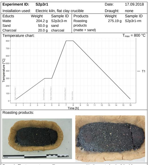
Remark: The temperature profile was programmed in the control unit of the kiln. Photos: © DBM/LEA, Erica Hanning
