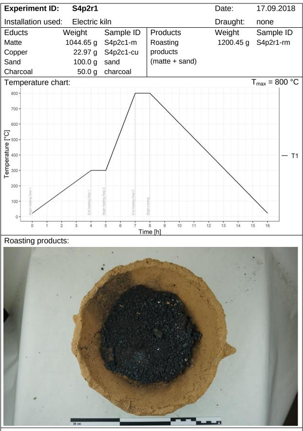
Remark: The temperature profile was programmed in the control unit of the kiln.
