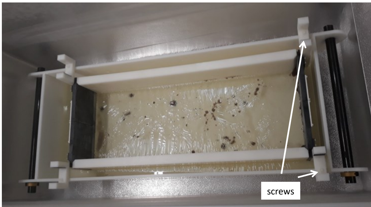
Figure 13. Syrup in the basin, with the inner sidewalls hanging in it. Note the dark material, which is leftover viscous material from a previous model. The inner sidewalls are fixed in place (i.e. by screws to the syrup basin), and the syrup is frozen, causing a subtle wrinkling on its surface.
