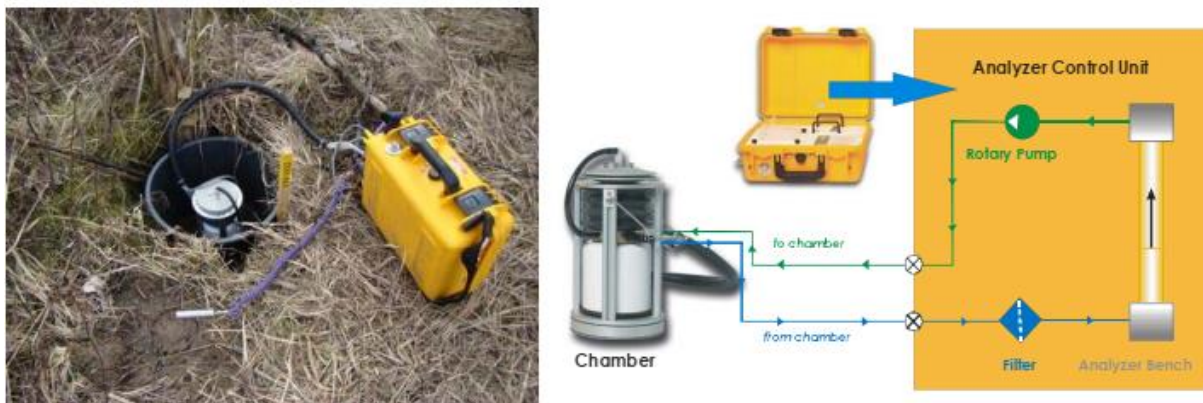
Figure 2: Field application and schematics of the automated soil CO 2 flux measurement system LI-8100 (LI-COR Biosciences)
