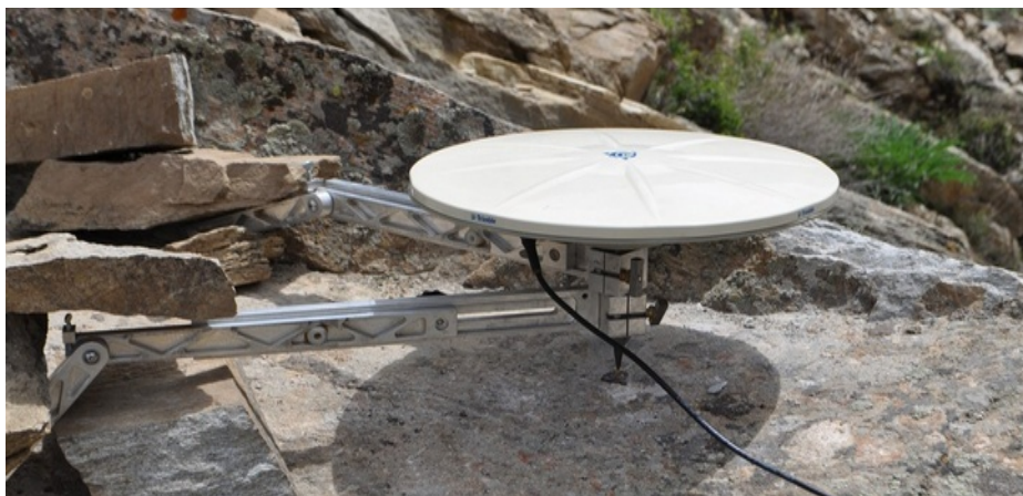
Figure 7: Typical GNSS antenna set up in Afghanistan, using a short-braced spike mount with a fixed height.
