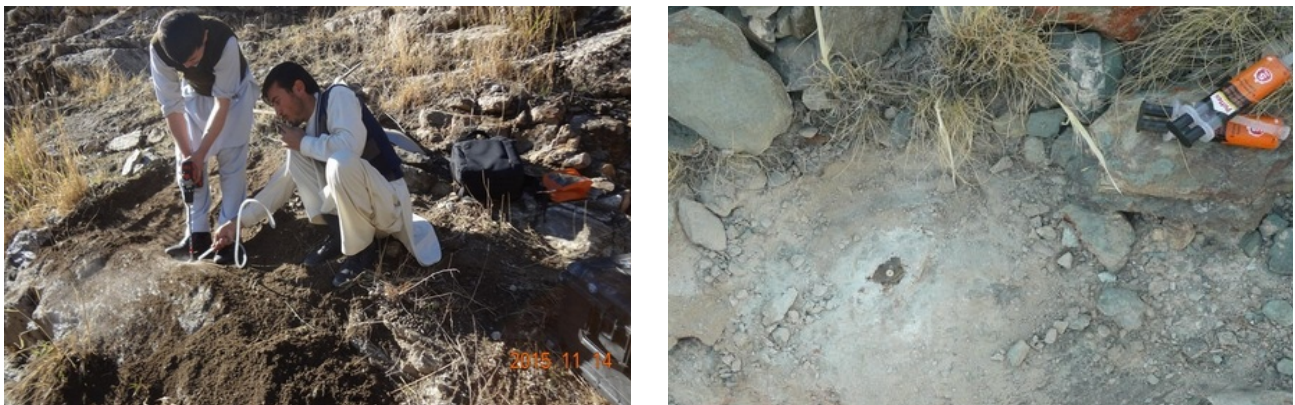
Figure 4: Installation of a stain-less steel bolt drilled (left) and glued (right) into unscattered bedrock.
