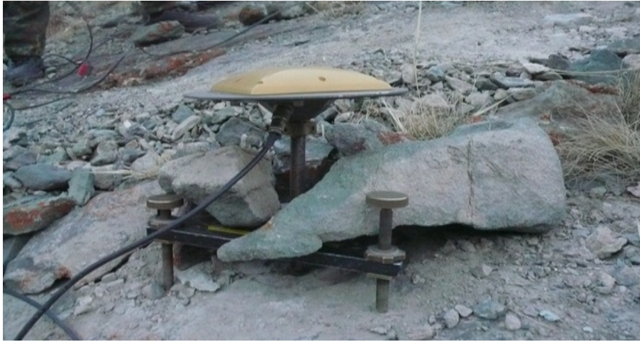
Figure 6: Typical GNSS antenna set up in Kyrgyzstan, using a three-legged adjustment table with a central spike mount, which was sometimes difficult to stabilize.
